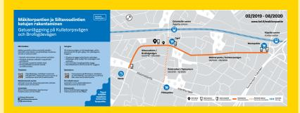
Pedestrian junctions should have a worksite information board installed at a readable level. In addition to the worksite information, the horizontal board should include a map, adjusted to the terrain's direction, which shows the current location with the 'You are here' dot. The map will also include the pedestrian and cycling paths, distances to key destinations in metres and minutes, key landmarks, and an arrow pointing north.
